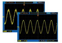
Filter out unwanted signal components such as various types of noise with built-in digital filters. Choose from Low-Pass, High-Pass, Band-Pass, and Band-Stop filters.
