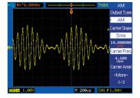
The built-in arbitrary waveform generator is capable of many different types of modulation for various applications. Modulate your waveforms with AM, FM, FSK, PSK, and PWM modulation schemes and use any of the 30 built-in waveforms as the modulating waveform. Multiple Ways to Interface
